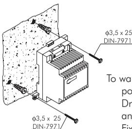
Install the transformer in a dry and protected place.
